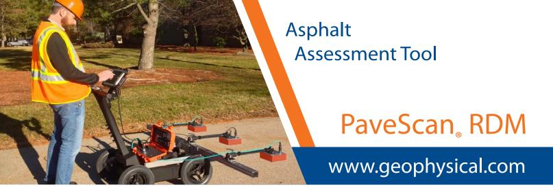
Problems that occur during the paving process, such as poor uniformity and significant variations in density, can result in premature failures. These failures include road raveling, cracking and deterioration along joints. The PaveScan RDM system provides accurate real-time measurements to ensure the life and quality of the pavement.
