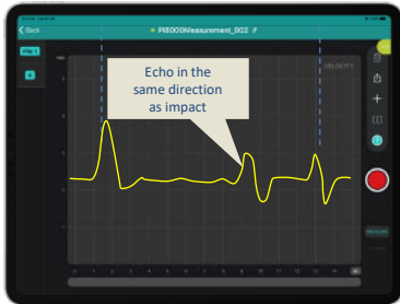
Necking – reduction in diameter
