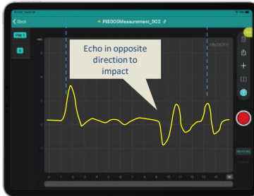
Bulging – increase in diameter
